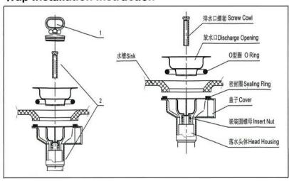
Note: The waste is fitted to 40mm bottle trap which shall be ordered separately
